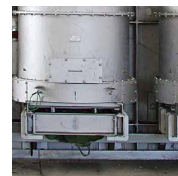
RegClean® (Option) Cleaning system for regenerators
