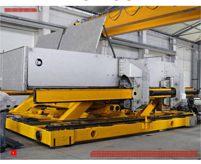
Movable – for charging contaminated scrap to hearth and multi-chamber melting furnaces with closed charging trough and hood
